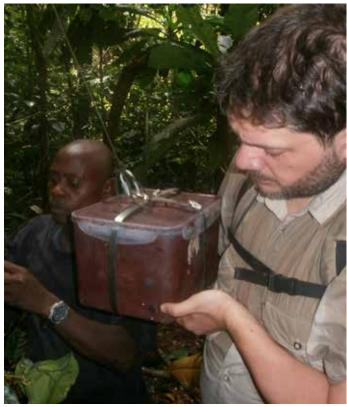
Setting up one of the Autonomous Recording Units (ARUs) used to monitor gunshots, Credit: WildCRU
